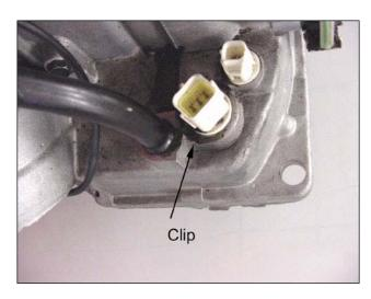
9. Remove the oil temperature sensor from the bracket. Remove the oil filter. Remove ten 10 mm bolts and remove the valve body.
