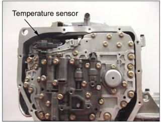
10. Remove the solenoids and carefully reinstall the new solenoids in the same location. Tighten the bolts to 3-4 lb-ft (40-60 kg.cm).
