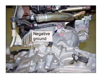
4. Clean the connection between the negative battery cable and the body ground bolt located next to the battery. Apply conductive grease to the connection before reinstalling the bolt.
