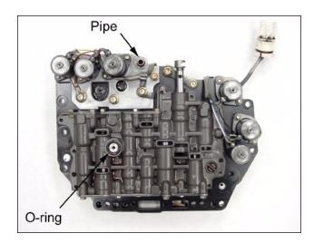
12. Carefully align the manual valve on the valve body to the manual control shaft and reinstall the valve body. Install the bolts and torque to 7-9 lb.ft (100-120 kg.cm).
